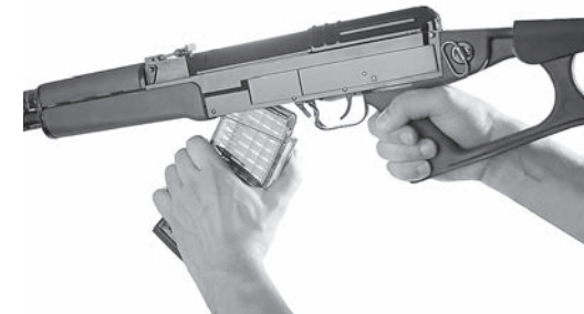
Fig. 27 Taking out the magazine
