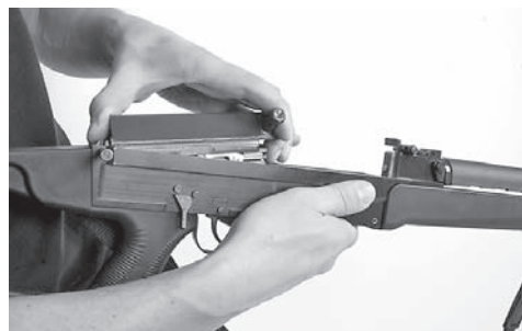
Fig. 29 Taking out the bolt
