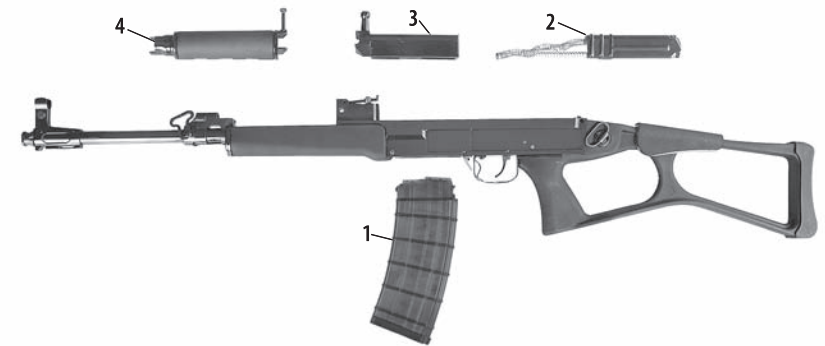
Fig. 26 The Sa vz. 58 Bolt action partially disassembled 1. Magazine, 2. Return mechanism, 3. Bolt, 4. Front guards
