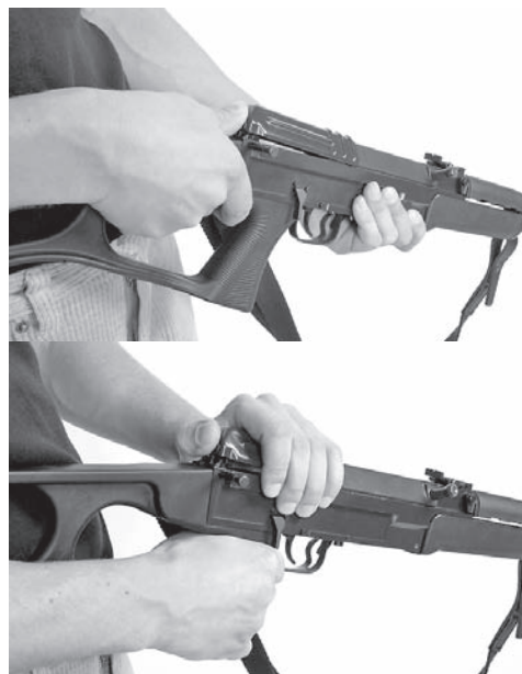
Fig. 28 Removing the return mechanism
