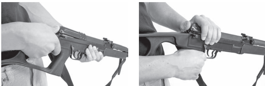
Fig. 28 Removing the return mechanism
