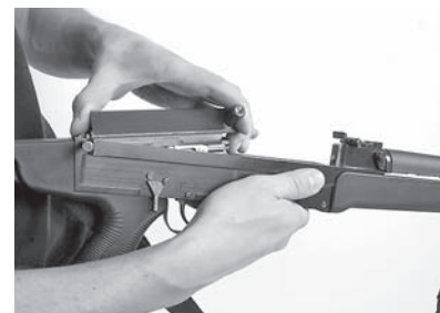
Fig. 29 Taking out the bolt
