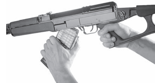
Fig. 27 Taking out the magazine
