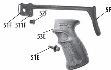
Fig. 19b Metal folding stock with grip 5F - Folding stock, 51F - Suspension of the folding stock, 511F - hinge of the folding stock, 52F - Folding stock screw, 53E - Ergonomic grip, 531E - Ergonomic grip screw
