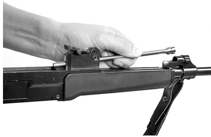
Fig. 30 Removing the piston
