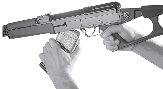
Fig. 27 Taking out the magazine
