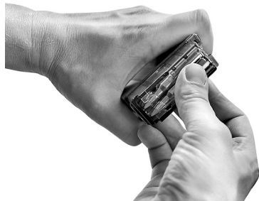
Fig. 24 - Loading the magazine
