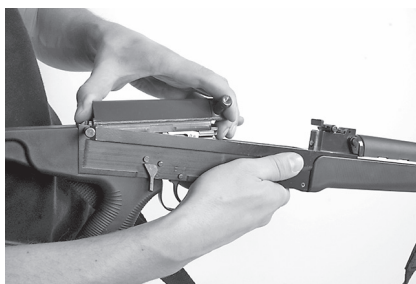
Fig. 29 Taking out the bolt
